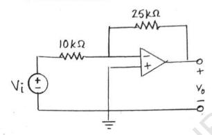
38. Find the output voltages of the Opamp inverting adder for the sets of input voltages and resistors shown in the figure.
