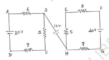
28. Using Thevenin theorem, calculate the current flowing through the load resistor  $R_L = 5\Omega$ .
