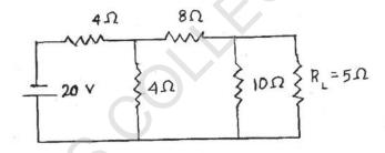
29. Calculate the value of R which will absorb maximum power from the following circuit. Also, compute the value of maximum power.
