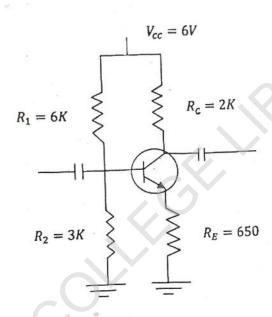
Calculate the emitter bias current for the transistor amplifier circuit shown in above figure.
